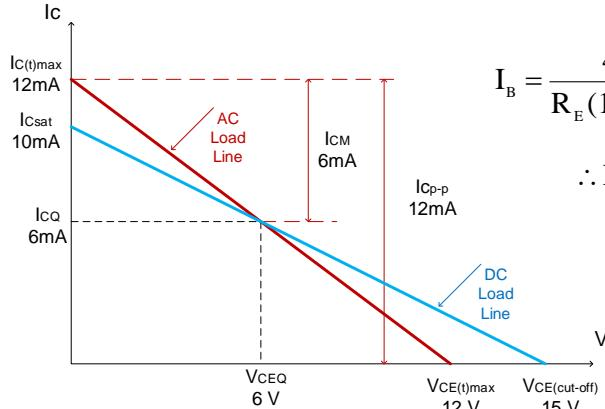
$$I_B = \frac{4.7 - 0.7}{R_E(100+1) + R_B} = \frac{I_{CQ}}{100} = 60 \mu\text{A}$$
