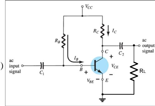
$$I_B = \frac{V_{CC} - V_{BE}}{R_B} = \frac{18 - 0.65}{576 \text{ k}\Omega} = 30 \mu\text{A}$$
