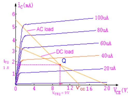
$$v_{ce} = -i_c(R_C // R_L) = -i_c R_L$$
