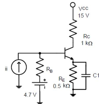
$$R_{ac} = R_C = 1 \text{ k}\Omega$$
