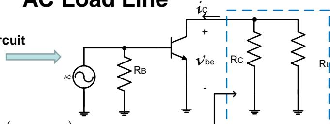
$$(V_{CE}(t) - V_{CEQ}) = -R_{ac} (I_C(t) - I_{CQ})$$
